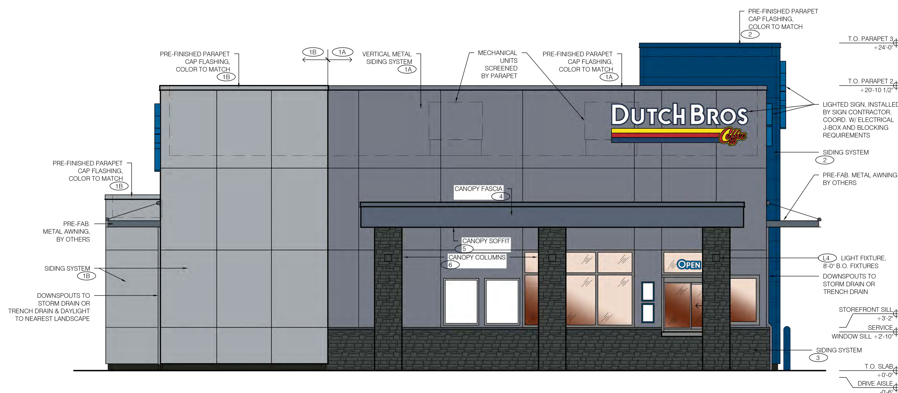
4 LEFT ELEVATION - DRIVE-THRU WINDOW
